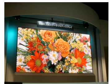
Fig.2 155-inch display with Seamless Tiling of OLED
