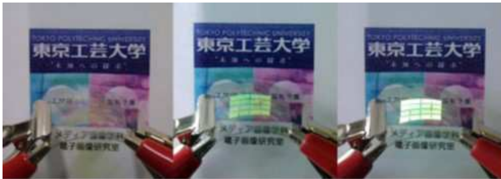
Fig.1 Flexible and transparent OLED.
