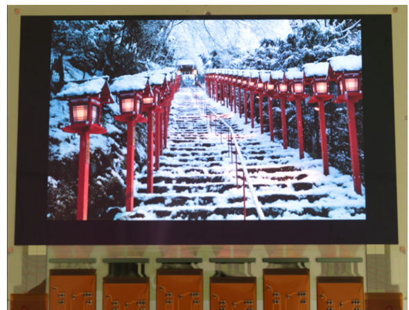
Figure 1. 1058-ppi 8.3-inch 8K OLED display with a crystalline oxide semiconductor backplane.
